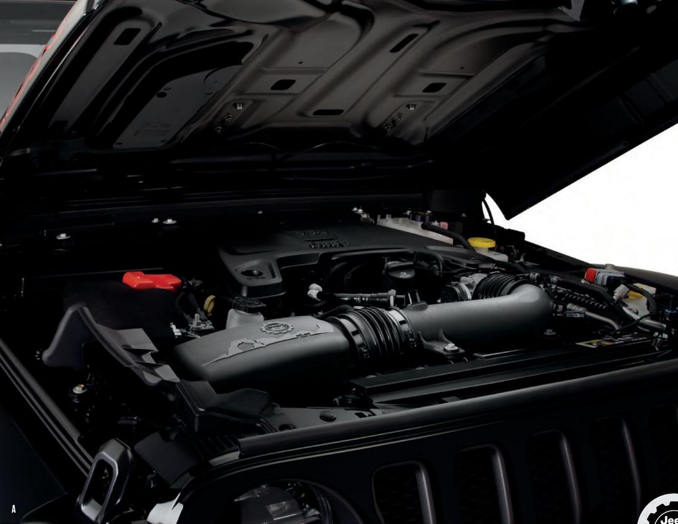
**A. COLD AIR INTAKE SYSTEM.<sup>(1)</sup>** Features Jeep® Performance Parts logo and reusable black and silver drop-in filter. Draws fresh air from outside vehicle into hood cutout to increase engine performance. Available for 3.6L engines only and includes bezel to finish cutout. [77072433AC]
