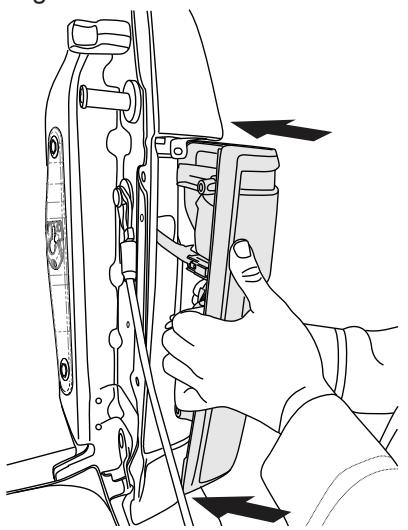
Torque top lamp fastener to 5.4 Ft-lbs/0.9 Nm.
