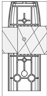
**NOTE:** The inside of the upright is stepped to fit correctly around the small and large diameter tubes.
