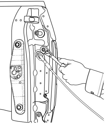
Torque bottom lamp fastener to 5.4 Ft-lbs/0.9 Nm.
