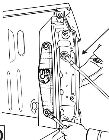
**NOTE:** Make sure nuts are centered correctly over D-pillar hole inside lamp cavity.
