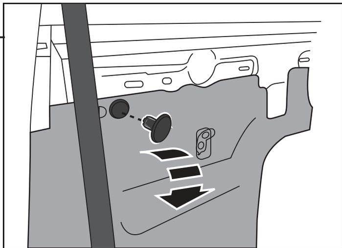
**34.** Remove the push-pin which secures the carpet backing and remove the carpet backing to expose metal surface of the cab. Retain the push pin and the carpet backing.
