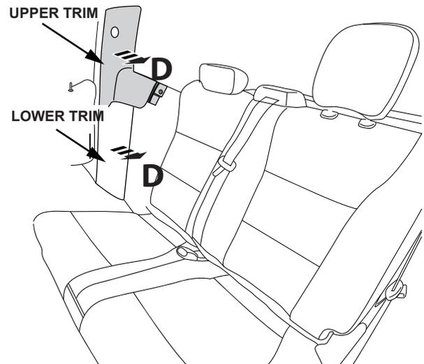
**23.** Remove the seatbelt first removing the seatbelt by unscrewing the T50 Torx bolt. Then remove the upper trim by removing the push pin. The lower pillar trim should also be removed at this time.
