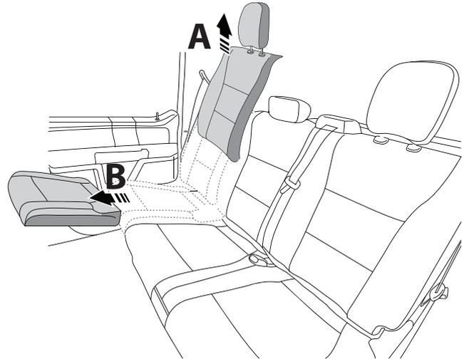
**22.** Remove the passenger side seat by unscrewing and removing the T50 Torx bolt on the top of the seat back and pull up on the seat back. The lower seat can then be removed by pulling the tab on the front of the seat and pushing the seat bottom back and lifting out.
