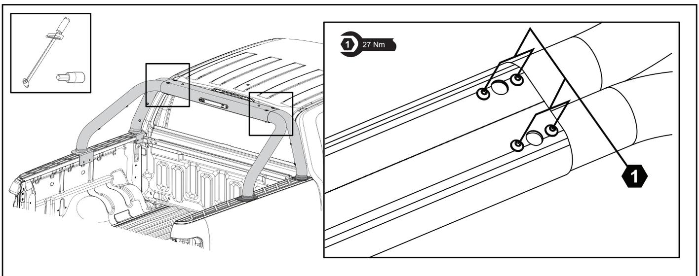
**19.** Fully tighten all 8 Leg to center piece bolts (1) to 27 Nm.
