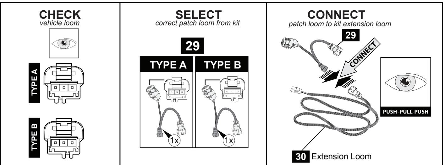
**26.** Check the keyway on the vehicle loom, it will be Type A or Type B as shown. Discard the Sportsbar Vehicle Patch (29) loom that does not have the same keyway type as your vehicle. Connect the correct Vehicle Patch loom (29) to the extension loom (30)
