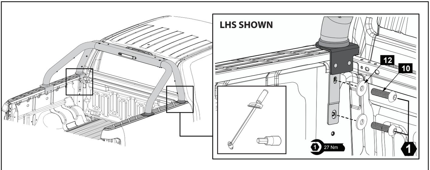
**17.** Attach the front foot brackets to the vehicle tub using screws (10) and washers (12). Tighten to 27 Nm.
