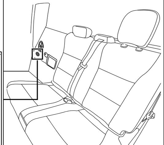
**24.** Locate the rubber grommet in the back of the back of the cab and pull it out and retain as it will be re-inserted in step 28.
