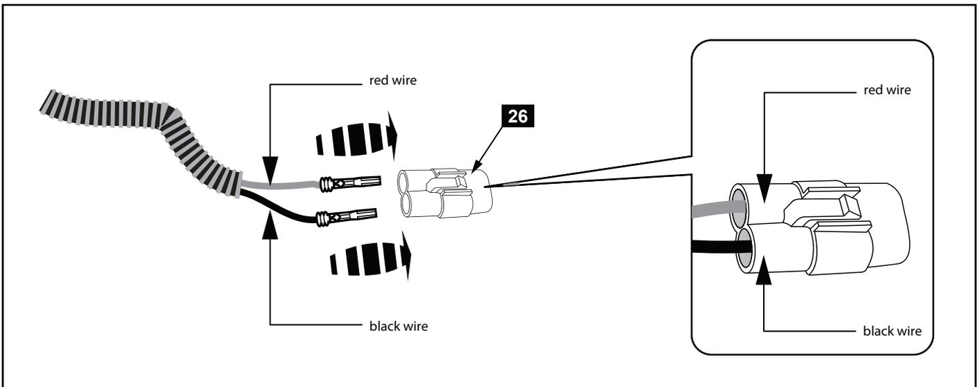
8. Remove the Stop Lamp Loom Plug (26) from the fitting kit. Push the red and black wires from the Stop Lamp Wiring Loom into the Stop Lamp Loom Plug.
