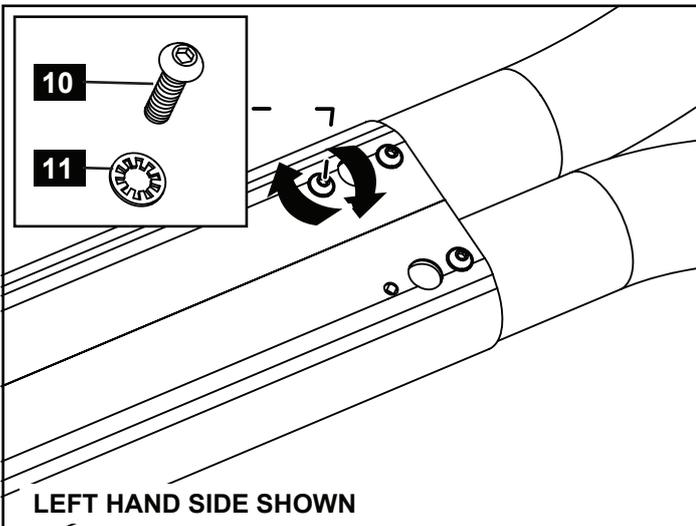
4. Install the remaining 2x M8 Pan HeadHex Screws (10) and M8 Internal Lock Washers (11) at each side. Do not fully tighten the screws.
