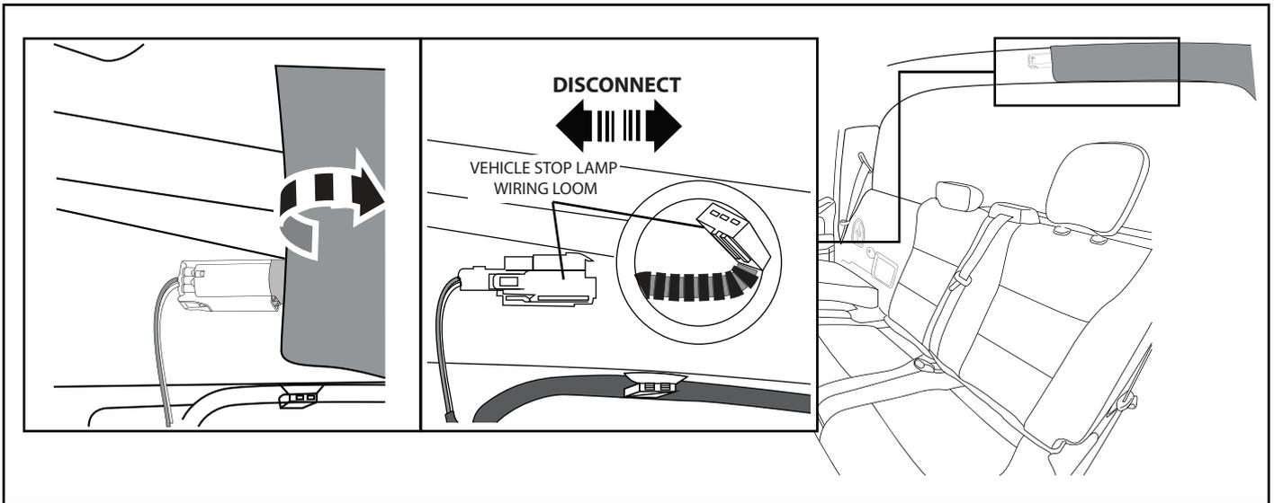
**25.** Lower the roof headliner directly opposite the rear Center high mounted stoplight (3rd stoplight). Locate the connector and disconnect.
