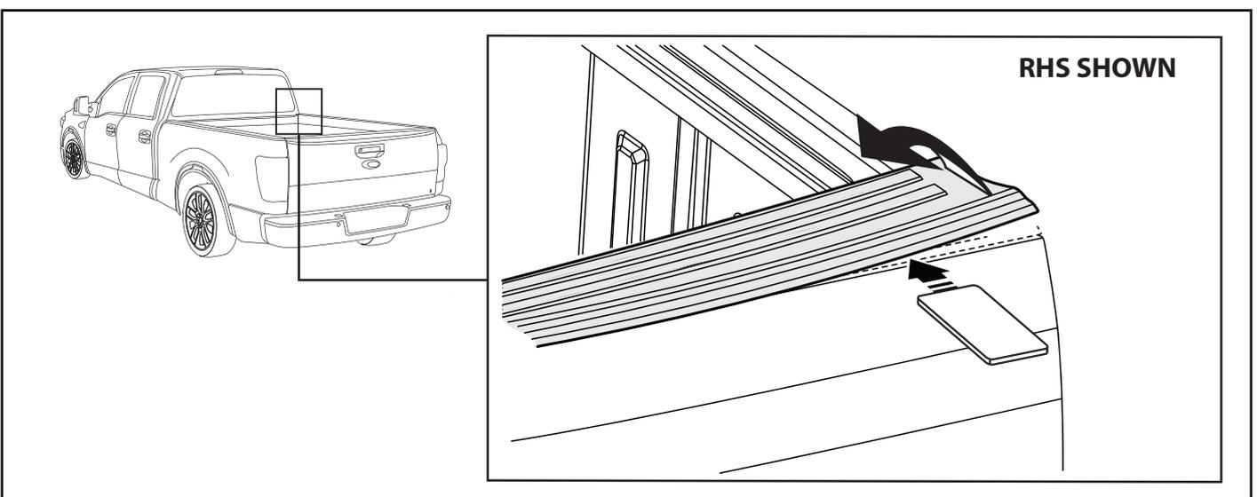
10. Carefully lift up the end of the bed rail cap upwards to disengage the clips. Place the rectangular foam block from the sports bar packaging underneath the bed rail cap to hold it in position above the bedrail.
