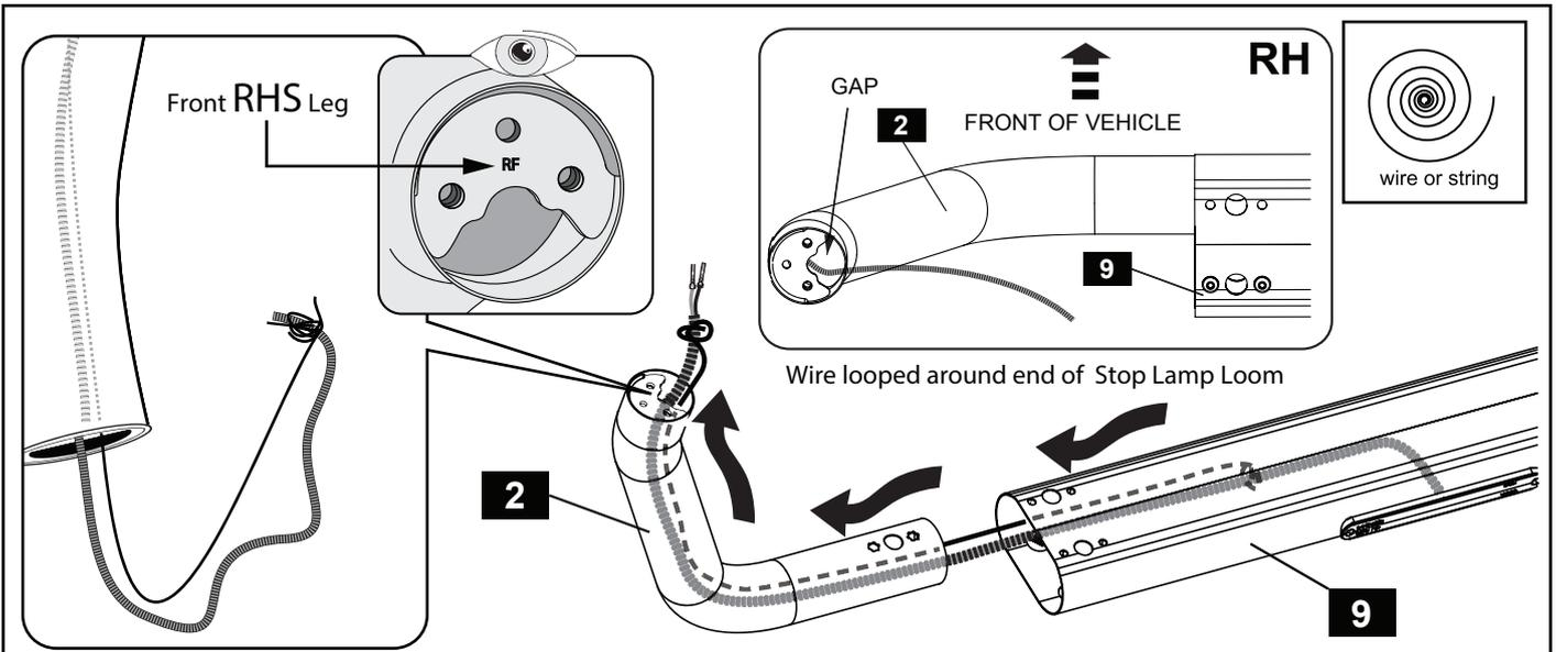
1. Place the center piece (9) on a soft surface so that the side with six holes per side is facing up (this is the underside of the part). Locate the Stop Lamp Wiring Loom inside the center piece (9) and pull through as shown. Insert a wire or piece of string through the gap in the foot of the RHS Front Leg (RF) (1), and use this to pull the stop lamp loom through the leg.
