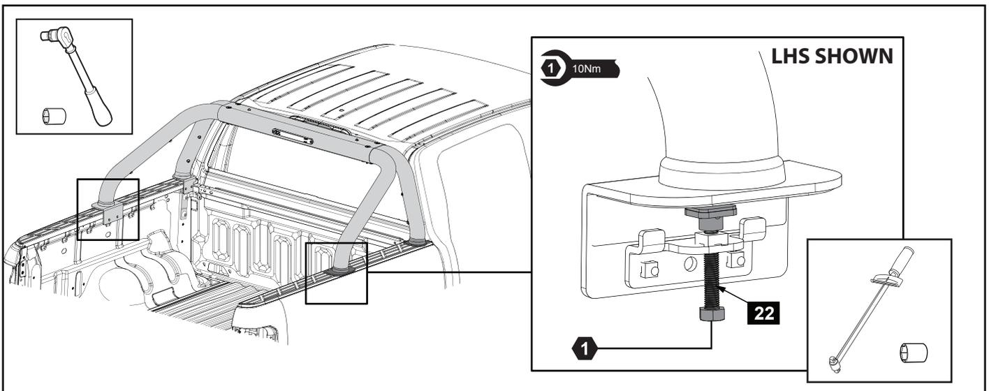
**18.** Tighten up the rear foot clamp plate bolts (22) to a torque of 10Nm. Repeat for the opposite side.
