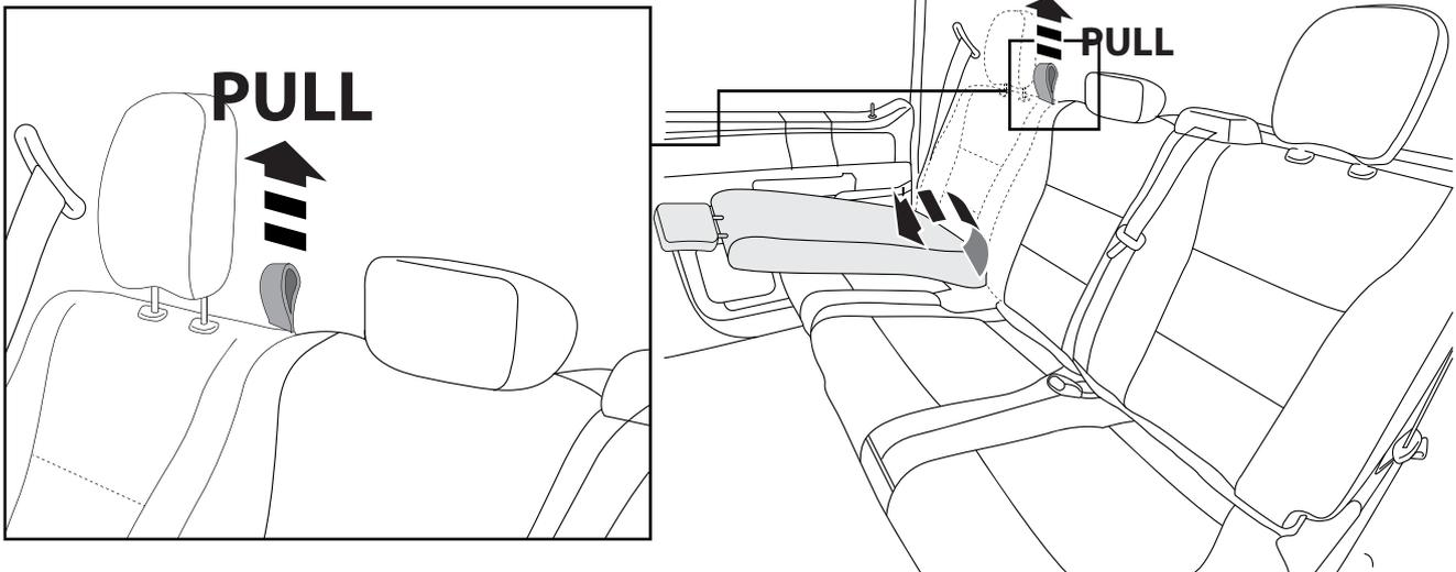
**32.** Lower the passenger rear seat by pulling on the loop on the side.
