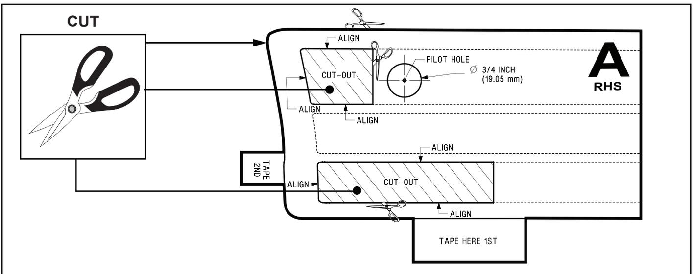
9. Cut out the outline of Paper Template A on Page 16AAa, and cut out the cross hatched guide 'cut-out' sections as marked.
