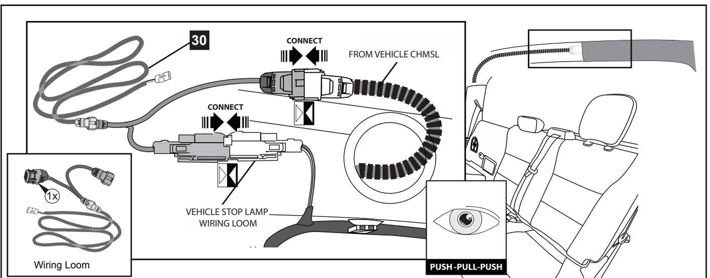
**27.** Plug both connectors on the T piece attached to the supplied loom in the kit (30) into the plug coming from the vehicle stop lamp loom. Tuck plug connection back under the headliner and feed the loom across to the passenger side pillar.
