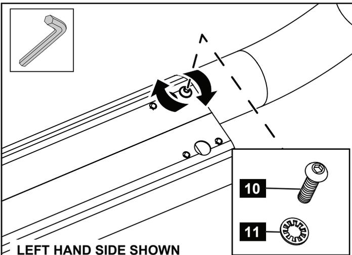
2. Take the RHS Front Leg RF (2) & LHS Front Leg LF (1) and install into the forward half of the Center Piece. Fasten using M8 Pan Head Screws (10) and M8 Internal Lock Washers (11). Do not fully tighten screws.
