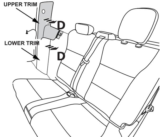
**33.** Remove the seatbelt first removing the seatbelt by unscrewing the T50 Torx bolt. Then remove the upper trim by removing the push pin. The lower pillar trim should also be removed at this time.
