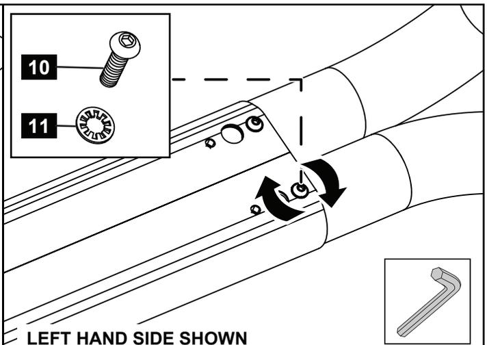
3. Take the RHS Rear Leg RR (4) & LHS Rear Leg LR (3) and install into the back half of the Center Piece. Fasten using M8 Pan Head Screws (10) and M8 Internal Lock Washers (11). Do not fully tighten screws.
