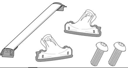
Place the front crossbar onto the roof rails. Orient using the front arrow molded on the underside of the crossbar.
