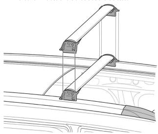
Adjust by sliding left stanchion outward to press against the left roof rail for a snug fit.
