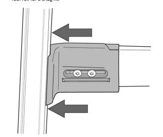
4 Install right clamp using clamp bolt and tighten to 9Nm using T27 torque tool.
