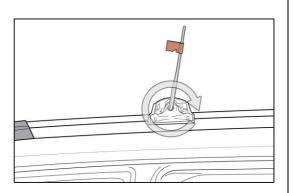
Attach tethers from the stanchions to the covers. Lower the end cap covers onto the crossbar and slide outward  $% \left( 1\right) =\left( 1\right) \left( 1\right)$ to engage the tangs. Rotate downwards to fully snap the covers into position.
