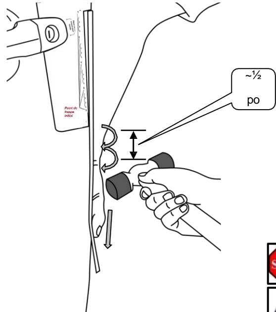
S'ASSURER QUE LA PROTECTION DE BORD DE PORTE EST COMPLÈTEMENT ENFONCÉE, PUIS FRAPPER EN REMONTANT VERS LE HAUT DE LA PROTECTION DE BORD DE PORTE.
