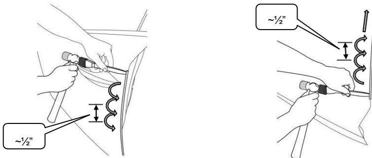
STARTING FROM EITHER THE TOP OR BOTTOM OF DOOR EDGE GUARD, LIGHTLY TAP NYLON REMOVAL TOOL ALONG GUARD EDGE IN 1/2" INTERVALS MOVING DOWN OR UP UNTIL ~2" OF DOOR EDGE GUARD IS DISENGAGED. REPEAT THIS PROCESS AT OTHER END. ONCE ~2" OF BOTH TOP AND BOTTOM OF DOOR EDGE GUARD IS DISENGAGED, CONTINUE UP OR DOWN ENTIRE DOOR EDGE GUARD LENGTH UNTIL REMOVAL IS COMPLETE.
