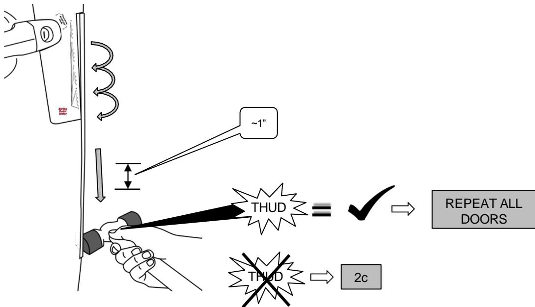
ONCE FULLY ENGAGED, PROGRESSIVELY TAP UP ENTIRE LENGTH OF DOOR EDGE GUARD. IF FULLY SEATED, A SOLID "THUD" SHOULD BE HEARD. IF NOT HEARD, REPEAT STEP 2c.
