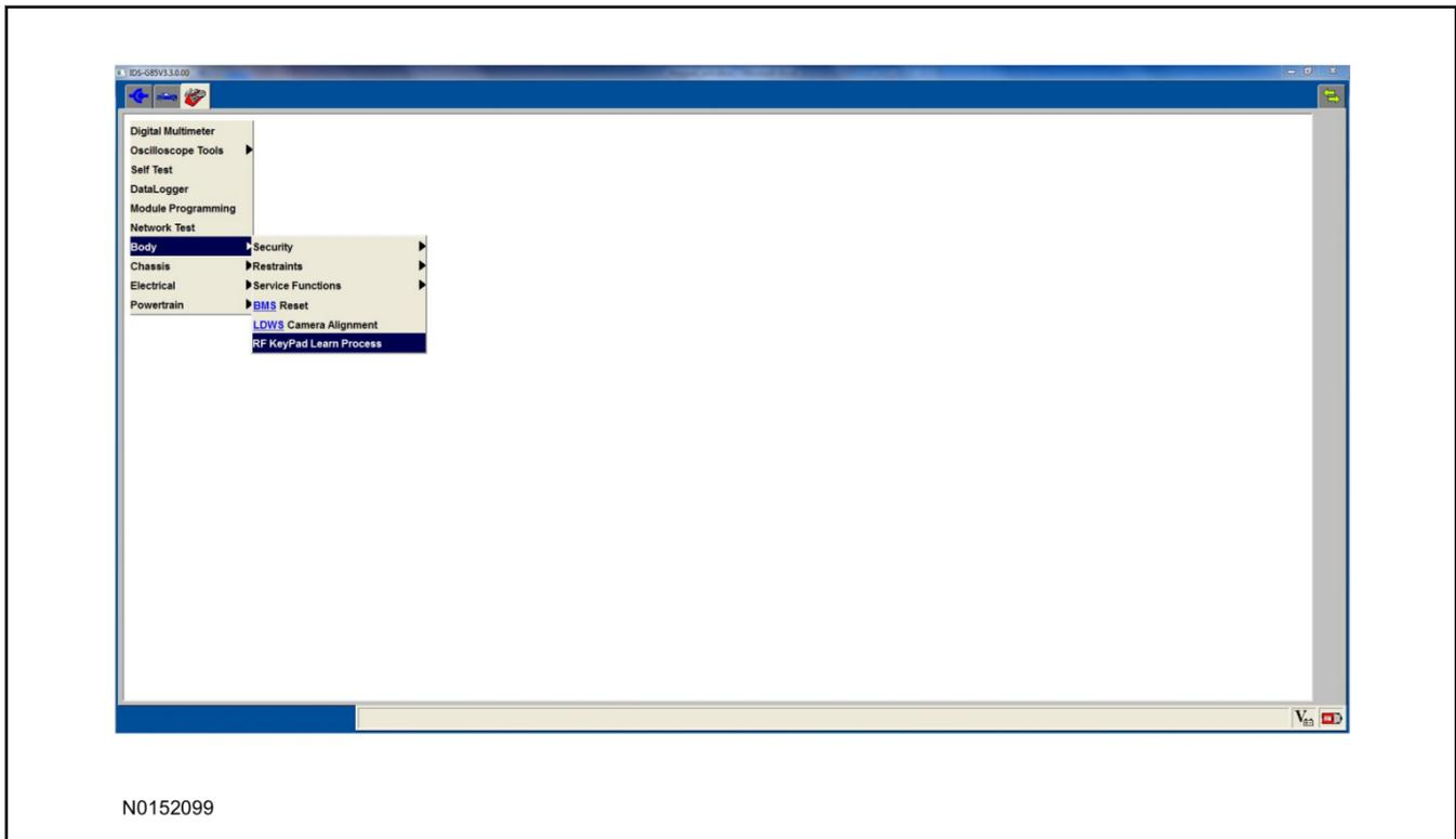
4. Program the keyless entry keypad to the vehicle using the FDRS.
