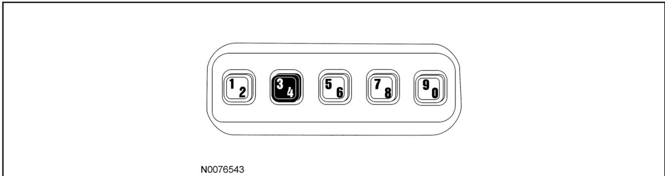
3. To unlock the trunk or hatch, if equipped, press the 5/6 button within five seconds of entering a valid keypad code (IKT vehicles may require the 5/6 button to be pressed twice). Press the 5/6 button twice to open or close the passenger side power sliding door, if equipped.
