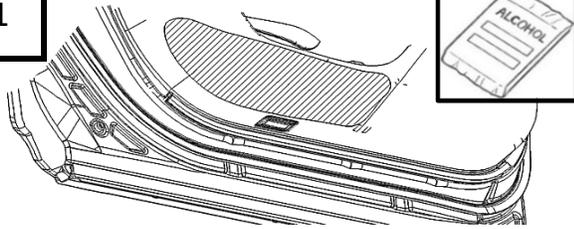
Clean driver's side front door in area shown above, first with soap and water, then with alcohol pad included. Allow time to dry.
