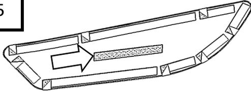
Remove adhesion tape backing from center
