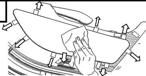
Remove adhesive backing tape by pulling out exposed tabs. Then apply pressure around Perimeter of Scuff protector to ensure proper adhesion to door
