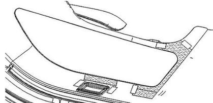
Remove installation templates and repeat process on passenger side by using backside of templates
