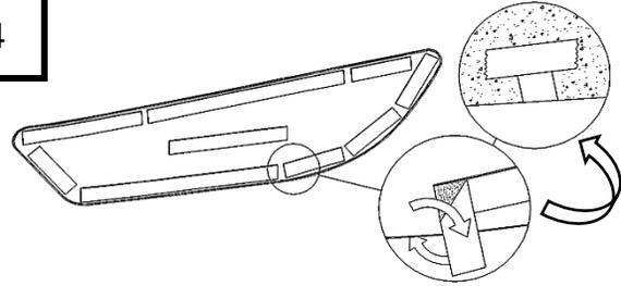
Fold over tabs on adhesion tape 45 degrees as shown and use tape to adhere tabs to front of protector in all 9 perimeter locations
