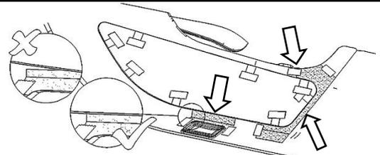
Align protector on door referencing speaker template, then door light template. Apply pressure in center to secure protector to door.
