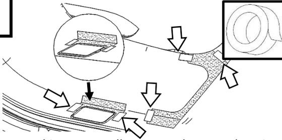
Using masking tape, adhere templates to door in the locations shown. Align to speaker grill, top of map pocket and door light as shown
