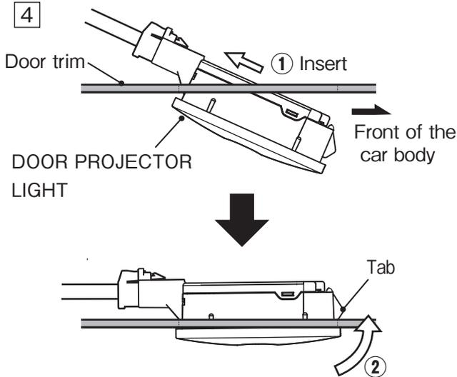
Insert the DOOR PROJECTOR LIGHT into the door trim. Ensure the front side tab is locked at the correct position. Repeat Steps 2 – 4 for the R Side Door.
