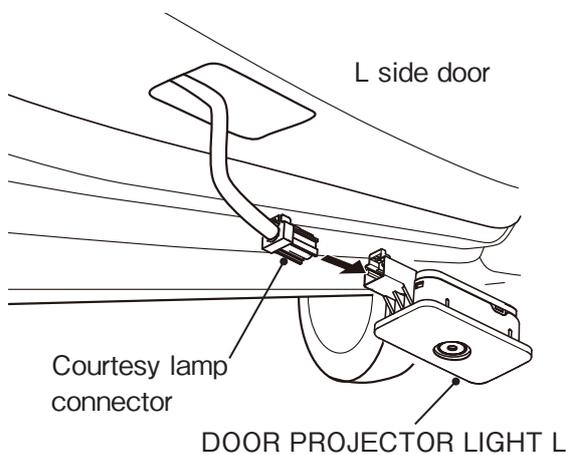
Confirm L/R side is correct. Connect the DOOR PROJECTOR LIGHT to the courtesy lamp connector.
