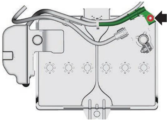
After removing the battery terminal, wait 60 seconds before proceeding to the next procedure.
