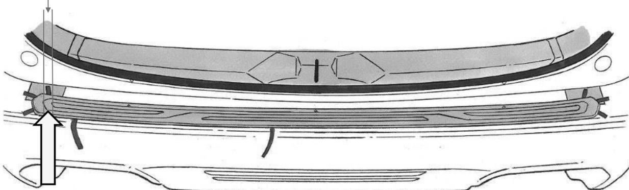
**STEP 17:** Carefully and gently remove the entire tape liner section shown below. Pulling with too much force or too quickly can tear the tape liner. **TIP:** If liner tears, pull the other liner that is intact.
