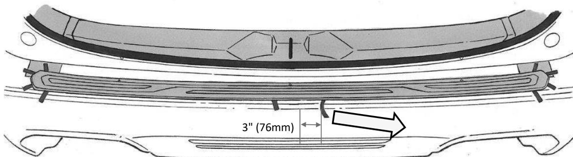
**STEP 8:** Press down on the part by a finger's width only at the location shown below. Do not press down anywhere else but now lightly hold the part in place.
