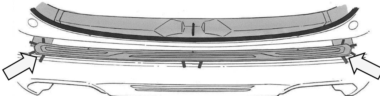
**STEP 7:** While firmly holding the part with your left hand, use your right hand to gently pull the liner shown below by approximately 3" (76mm) **BUT DO NOT PRESS DOWN.**
