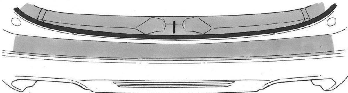
**STEP 2:** Note: If the temperature is below 60°F (15°C), heat the double sided tape and bumper surface to a temperature of 80°F (27°C).
