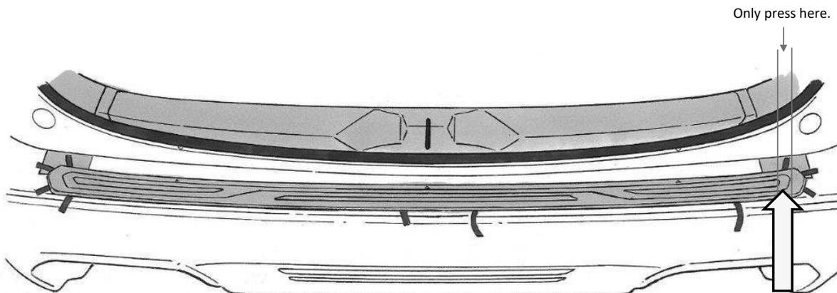
**STEP 11:** Carefully and gently remove the entire tape liner section shown below. Pulling with too much force or too quickly can tear the tape liner. **TIP:** If liner tears, pull the other liner that is intact.
