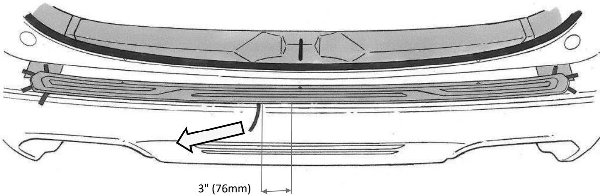
STEP 14: Press down on the part by a **finger's width** only at the location shown below. Do not press down anywhere else.
