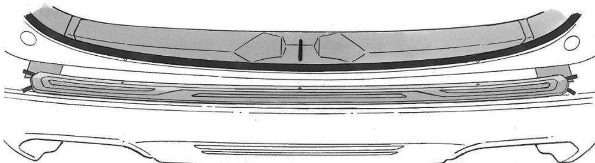
**STEP 21:** Carefully and gently remove the two tape liner sections shown below. Pulling with too much force or too quickly can tear the tape liner. **TIP:** If the liner tears, pull the same liner from the opposite direction. Then remove corner alignment templates.
