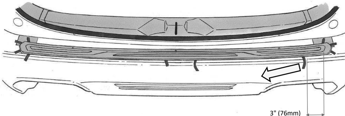
**STEP 10:** Carefully inspect and align (if necessary) the side of the part to the bumper and then press down on the part by a finger's width only at the location shown below. Do not press down anywhere else.
