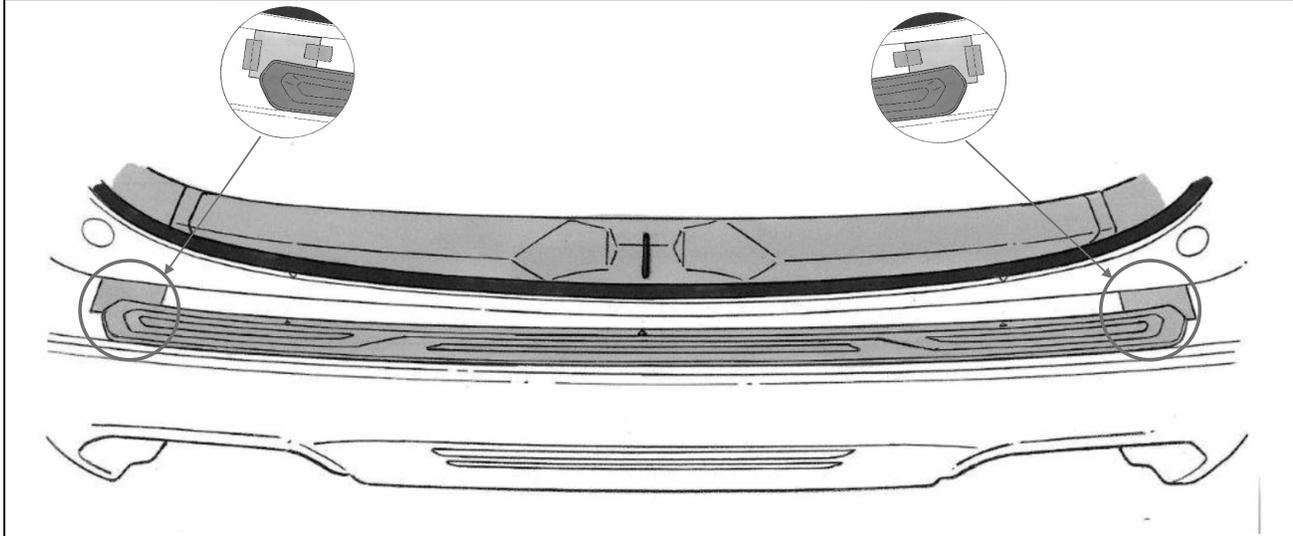
**STEP 5:** Flip part over. Fold and crease the tape liners as shown in the illustration below. You may tape each liner to the top surface of the part (optional).
