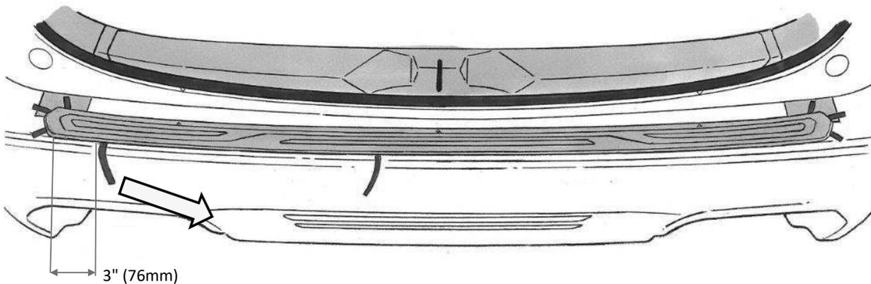
**STEP 16:** Carefully inspect and align (if necessary) the side of the part to the bumper and then press down on the part by a finger's width only at the location shown below. Do not press down anywhere else.
