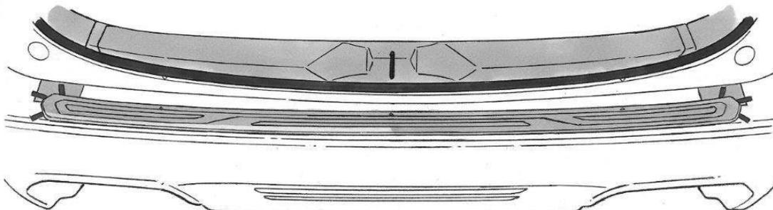
**STEP 19:** Carefully and gently remove the entire tape liner section shown below. Pulling with too much force or too quickly can tear the tape liner. **TIP:** If liner tears, pull the other liner that is intact.
