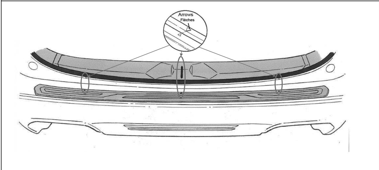
**STEP 4:** While part is in the home position locate supplied left and right corner alignment templates. Using the part as a guide position the right then the left templates. Ensure templates are against back vertical wall and aligned with part profile, then tape down outside edges of templates.
