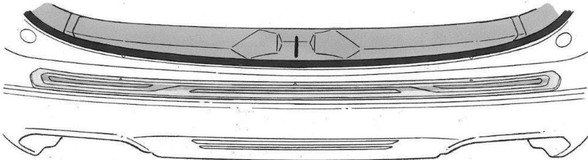
**STEP 23:** Inspect part for any areas not adhering to the bumper. Firmly pressed down as needed. Done.
