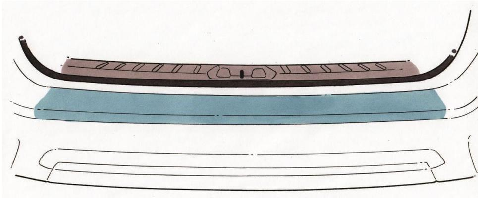
**STEP 2:** Note: If the temperature is below 60°F (15°C), heat the double sided tape and bumper surface to a temperature of 80°F (27°C).
