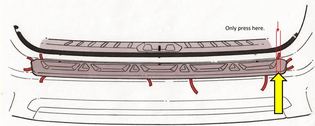
**STEP 10:** Carefully and gently remove the entire tape liner section shown below. Pulling with too much force or too quickly can tear the tape liner. **TIP:** If liner tears, pull the other liner that is intact.
