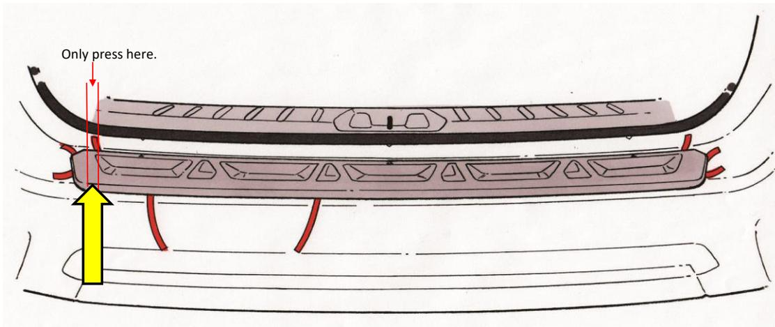
**STEP 16:** Carefully and gently remove the entire tape liner section shown below. Pulling with too much force or too quickly can tear the tape liner. **TIP:** If liner tears, pull the other liner that is intact.
