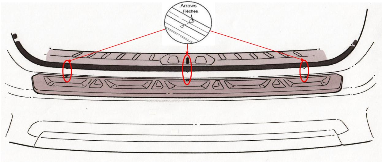
**STEP 4:** Flip part over. Fold and crease the tape liners as shown in the illustration below. You may tape each liner to the top surface of the part (optional).
