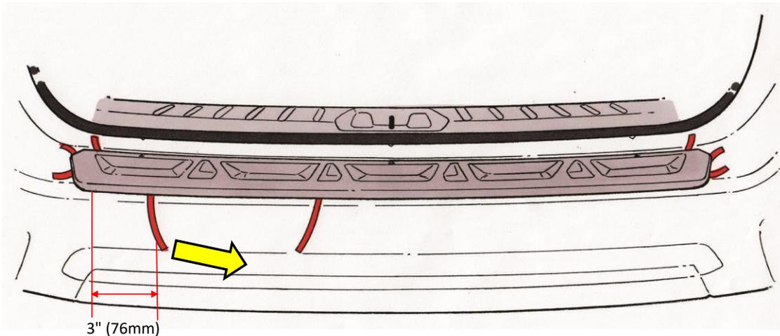
**STEP 15:** Carefully inspect and align (if necessary) the side of the part to the bumper and then press down on the part by a finger's width only at the location shown below. Do not press down anywhere else.
