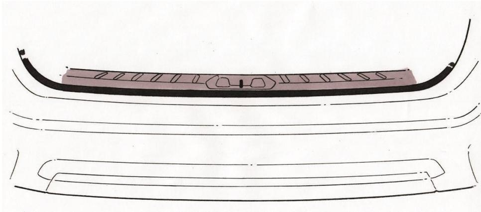
**STEP 1:** Clean any dirt, oil or wax from attaching area of bumper with a clean cloth and rubbing alcohol. Then prepare the surface with the supplied alcohol pads.
