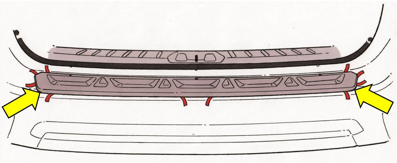
**STEP 6:** While firmly holding the part with your left hand, use your right hand to gently pull the liner shown below by approximately 3" (76mm) **BUT DO NOT PRESS DOWN.**
