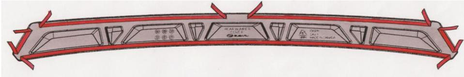
**STEP 5:** Reposition part onto rear bumper. Align again following STEP 3. Ensure each tape liner is positioned properly from STEP 4. Find the "home" position and inspect both sides of the part to ensure proper positioning then firmly hold part in place.
