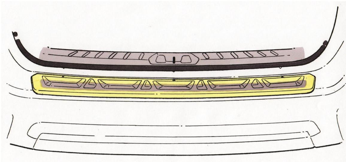
**STEP 22:** Inspect part for any areas not adhering to the bumper. Firmly pressed down as needed. Done.
