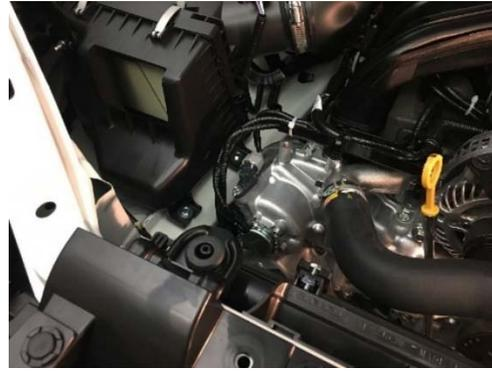
10. Feed orange block heater element connector through upper front grille air intake opening towards radiator. Using male plug protector, attach male plug to grille work as shown.
