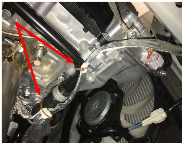
15. Plug harness into heater element. Orient orange connector towards the front by twisting the orange connector inside the heater body. The inside of heater can be rotated relative to the outer body.
