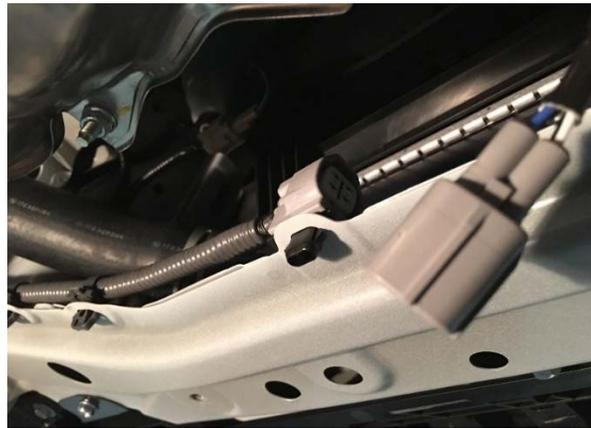
4. Carefully lower the front exhaust pipe by removing the 6 attachment nuts to gain access to the threaded core plug.
