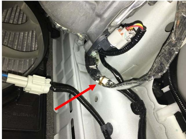
14. Attach harness to coolant pipe at the two locations shown by using 2 high temperature wire ties.
