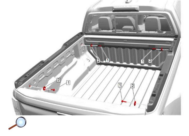
9. Install the M8 bolts (1) and washers (2) to the brackets. While pulling down on the bases tighten the M8 bolts (1) to 9 N.m (7 lb ft).
