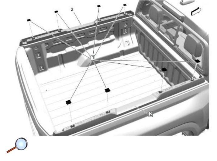
20. Install the cap covers (1) to the rails (2), making sure they snap into place.
