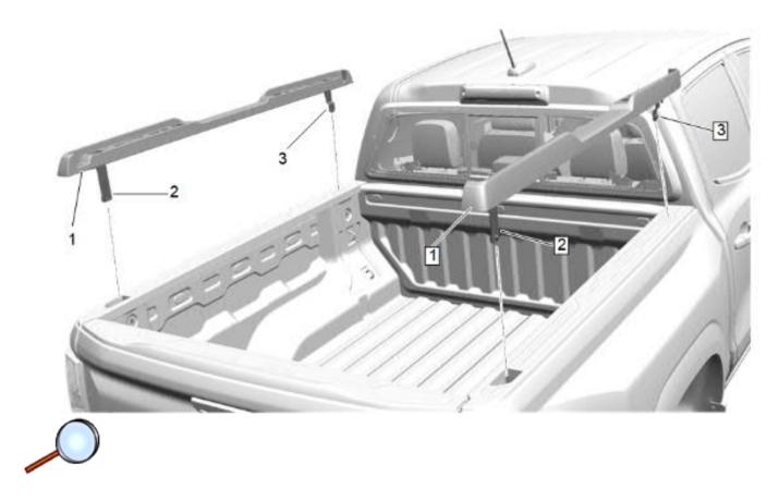
12. Remove the bases (1) with bracket (2), (3) from the vehicle.
