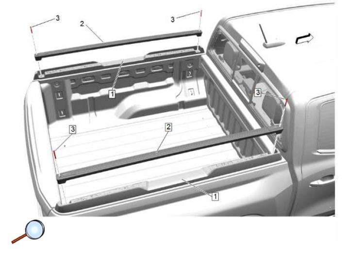
21. Place the cross rails (2) onto the base (1) in the stowed position. Secure the cross rails to the base with the countersunk M6 screws (3). Hand tighten the M6 screws with the supplied M6 hex key.
