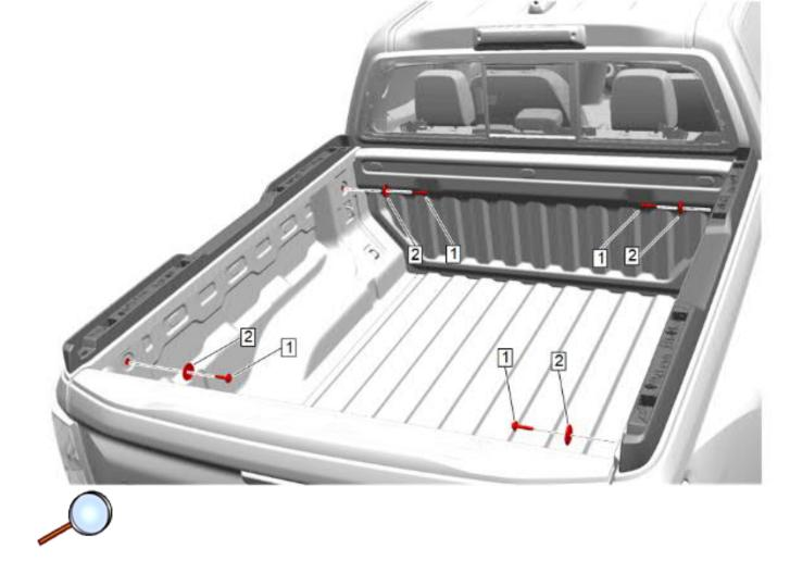
11. Remove the M8 bolts (1) and washers (2) from the brackets.
