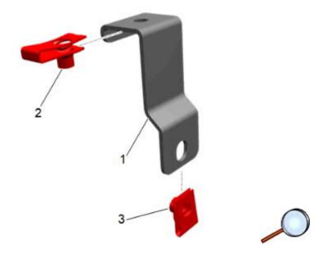
5. Assemble the front bracket (1). Using the wide range J-nut (2) for the top part of the bracket, and the narrow neck J-nut (3) for the bottom. Repeat step for other front bracket.
