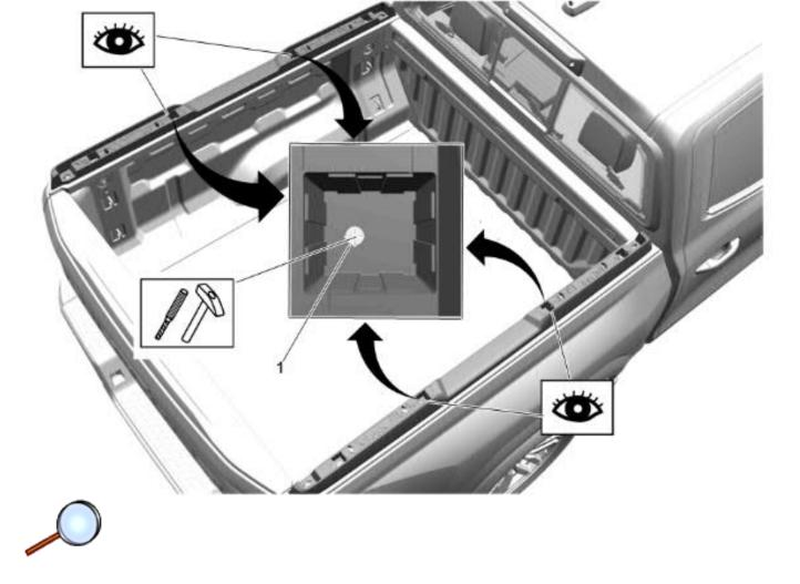
10. Identify the four locations (1) where part will mount to the pickup box. Center punch each location (1).
