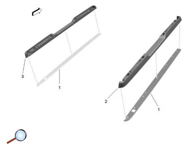
3. Install the base foam pieces (1), starting from one end to the middle and then install the second piece from the middle to end to the correct LH (3) and RH (2) bases.
