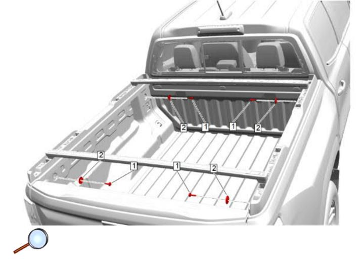
16. Install the M8 bolts (1) and washers (2) to the brackets. While pulling down on the bases tighten the M8 bolts (1) to 22 N.m (16 lb ft).
