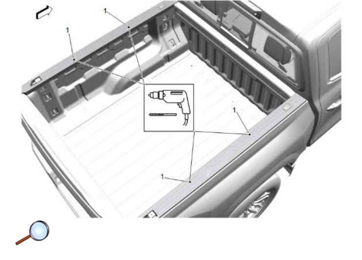
**Note:** Do not drill into the box with the rails on the vehicle.
