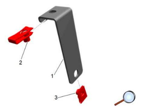
4. Assemble the rear bracket (1). Using the wide range J-nut (2) for the top part of the bracket, and the narrow neck J-nut (3) for the bottom. Repeat step for other rear bracket.
