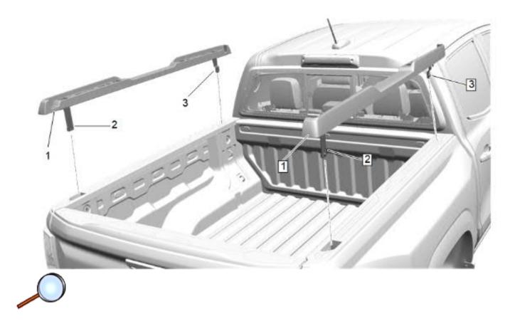
8. Place the bases (1) to the appropriate side of the vehicle making sure that the brackets (2), (3) are orientated correctly.
