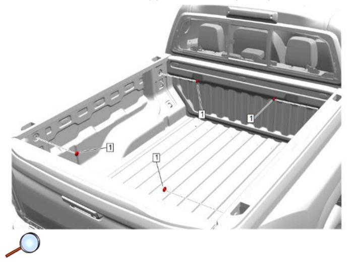
6. Remove the four rubber plugs (1) from the pickup box.
