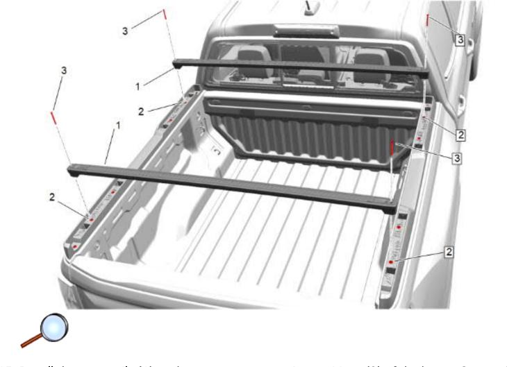
15. Install the cross rails (1) to the outer most mounting positions (2) of the bases. Secure the cross rails to the base with the countersunk M6 screws (3). Hand tighten the M6 screws with the supplied M6 hex key.
