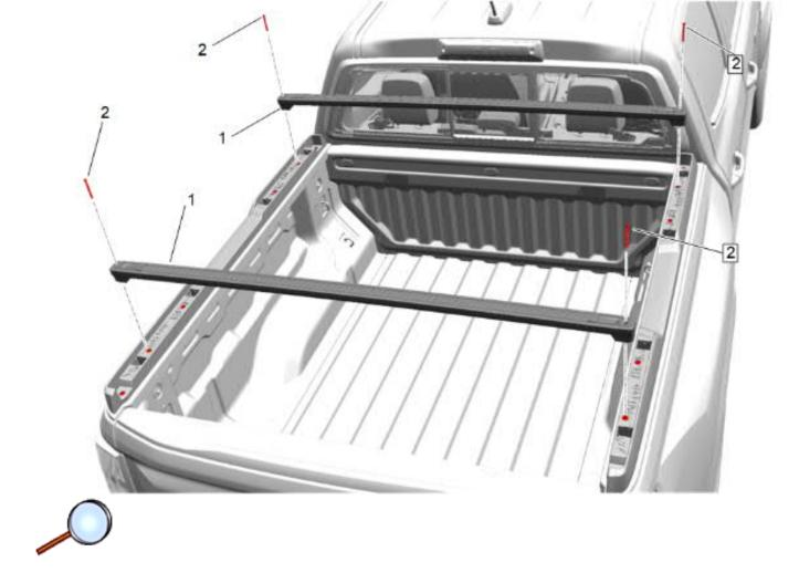
19. Remove the countersunk M6 screws (2) and cross rails (1) and set aside.
