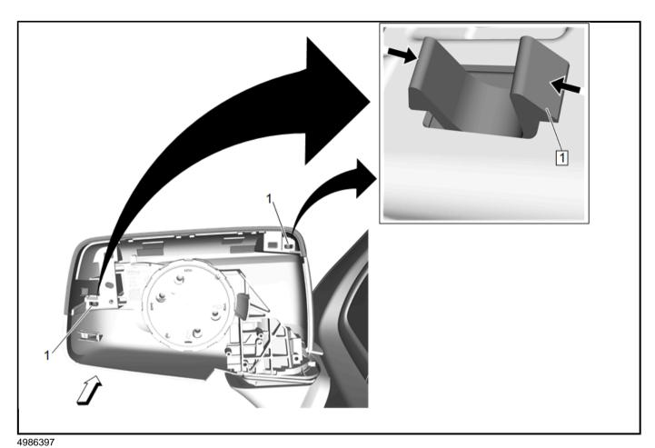
8. Depress the two retaining tabs (1) on the mirror cover.
