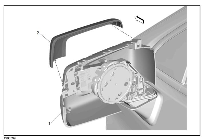
9. Grasp mirror housing cover (2) and lift outwards from the mirror housing (1) to release the retainers.
