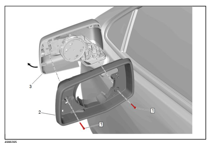
2. Install the bezel (2) to the mirror housing (3).
