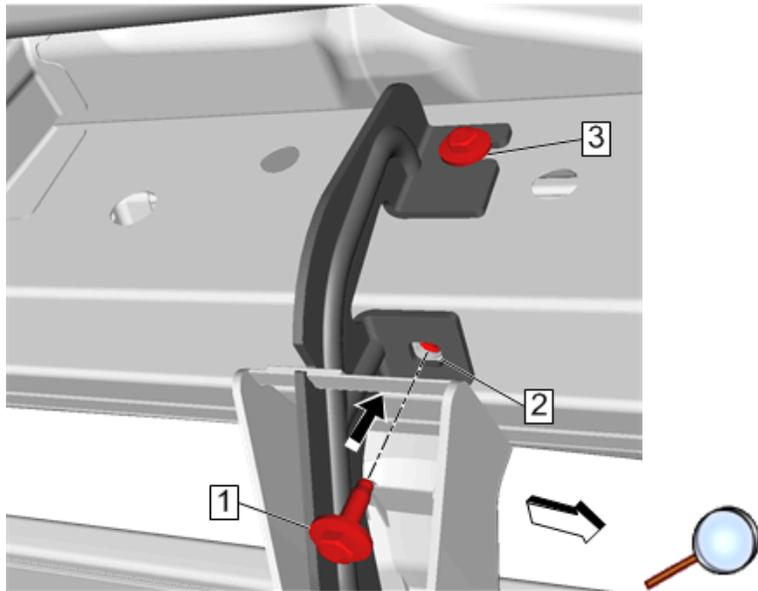
3. Insert the screws (1) in the horizontal mounting locations through the brackets (2). Adjust step fit and tighten screws to 22 N-m (16 lb ft). Tighten the screws (3) in the vertical mounting holes to 22 N-m (16 lb ft).
