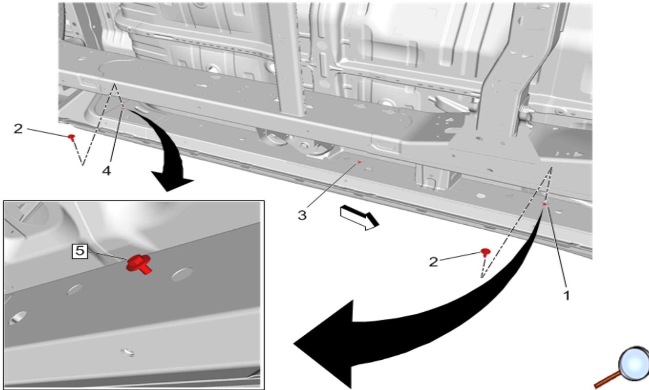
1. Locate the fore (1) and aft (4) mounting holes in the LH rockers. Insert screw (2) into fore and aft holes in the vertical surface of the rocker leaving the center locations (3) empty. Leave room for the bracket to fit over screws (5)
