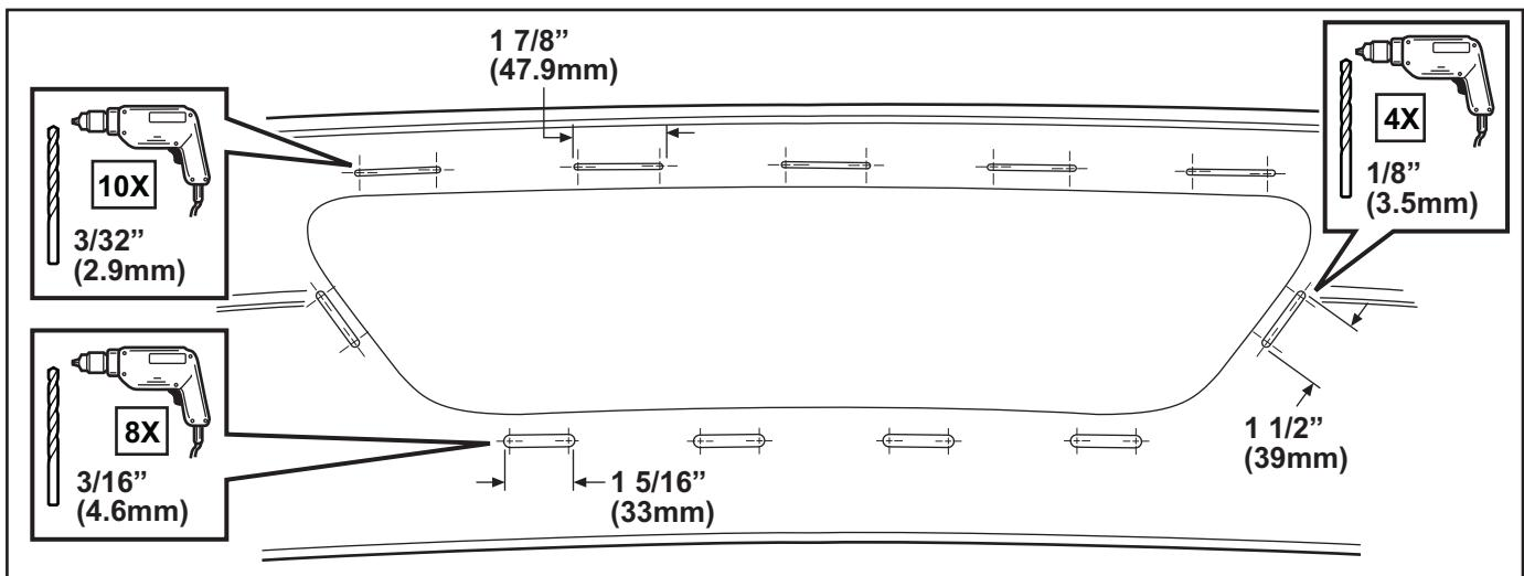
8. Cut through remaining areas of tab openings with a utility knife according to scribed areas as shown. Discard cut out portions.
