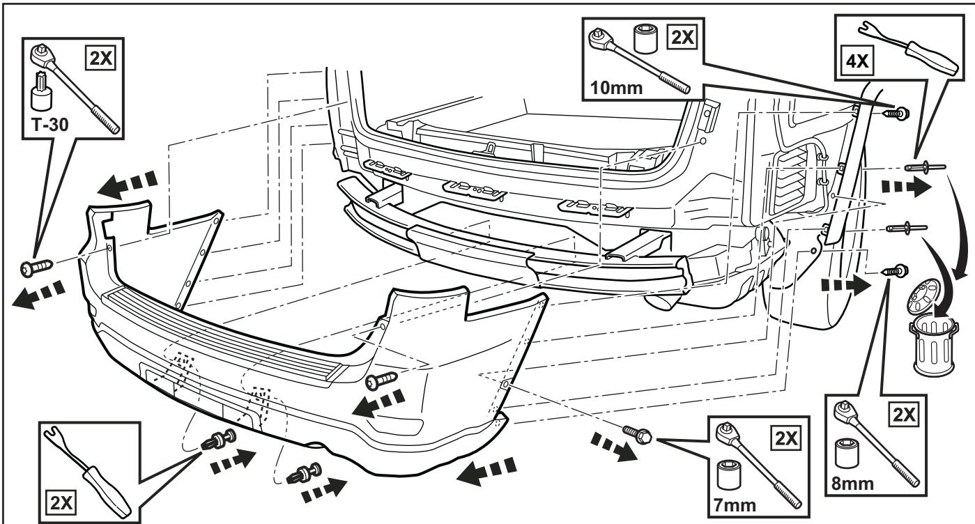
2. Unbolt and remove existing crossmember. Discard crossmember and all fasteners.
