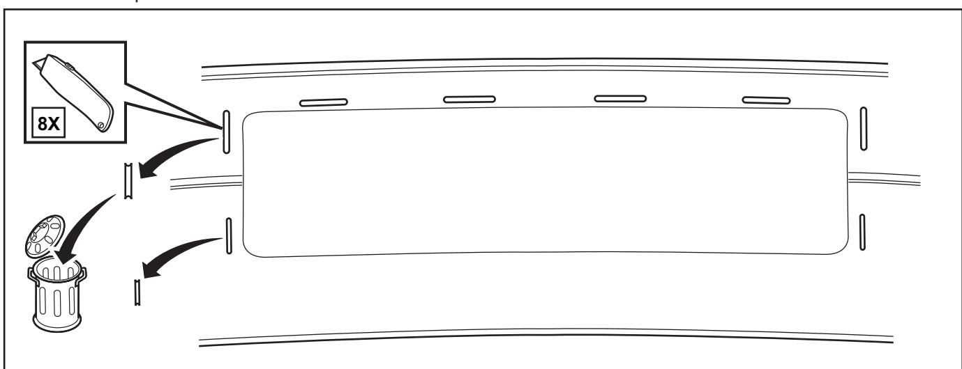
6. Cut out center bezel opening according to scribed areas as shown. Discard cut out portion.
