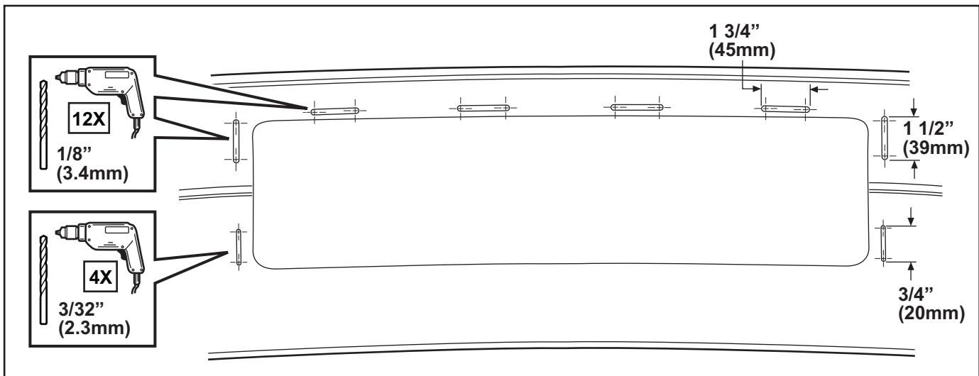
5. Cut through remaining areas of tab openings with a utility knife according to scribed areas as shown. Discard cut out portions.
