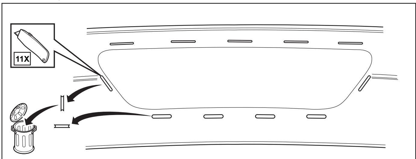
9. Cut out center bezel opening according to scribed areas as shown. Discard cut out portion.
