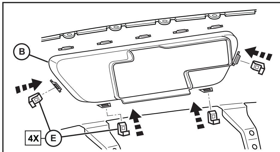
11. Using (8) 21mm bolts provided with the kit, install new hitch assembly. Tighten (8) bolts to 165 Nm (122 ft. lbs.).
