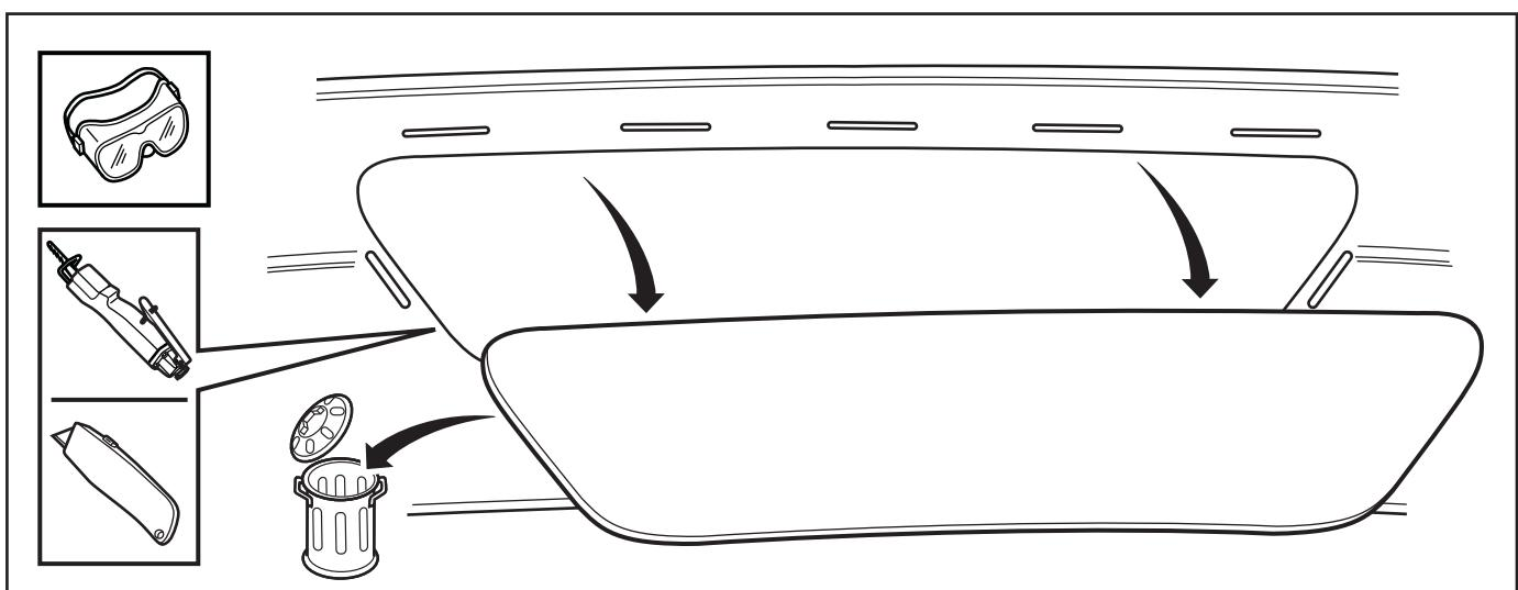
10. Press bezel into bumper opening. Be sure all tabs are firmly pressed in and secure with (2) spring clips as shown.
