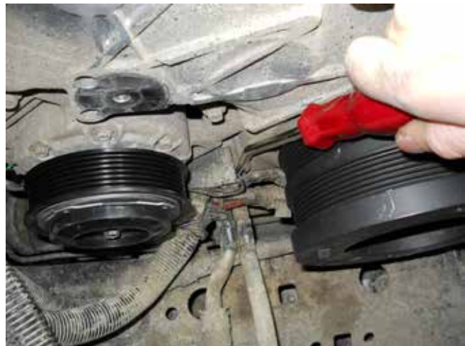
7. Remove the bolt. The line and wiring harness will need to be fastened to the tensioner bracket in a later step.
