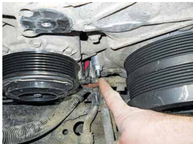
7. Remove the bolt. The line and wiring harness will need to be fastened to the tensioner bracket in a later step.
