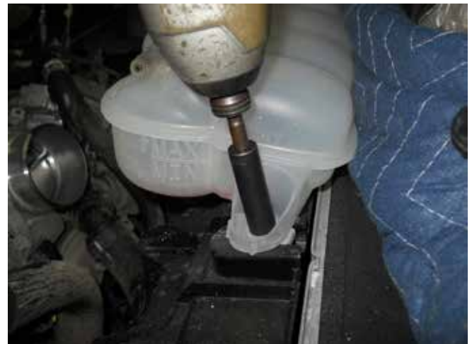
18. Remove two (2) mounting bolts.
