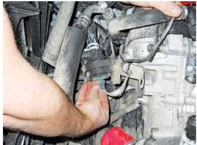
4. Pry the pump free from the retainer.
