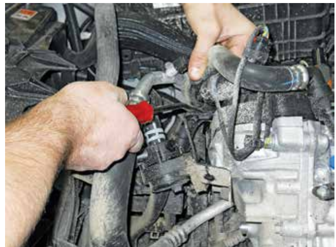
4. Pry the pump free from the retainer.
