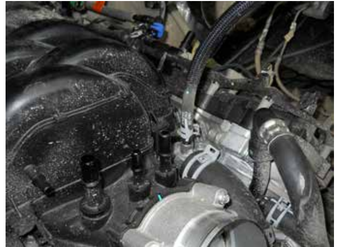
17. Disconnect degas upper bottle-to-radiator hose.
